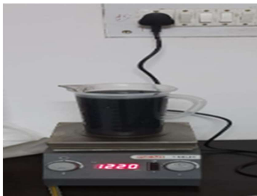
Figure 3 magnetic stirrer process for fuel preparation.
