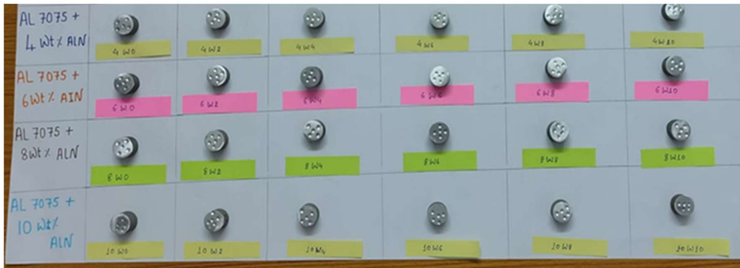
Figure1: The pictorial view of Hardness specimen before and after indentation
