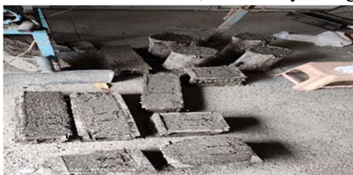
Figure 5: Casting of cubes, cylinders, and prisms
