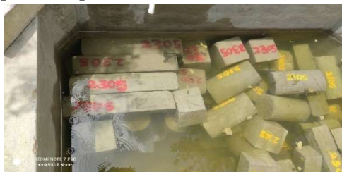
Figure 6: Curing of Specimens
