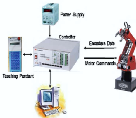
Figure (5) General System of The Robot
