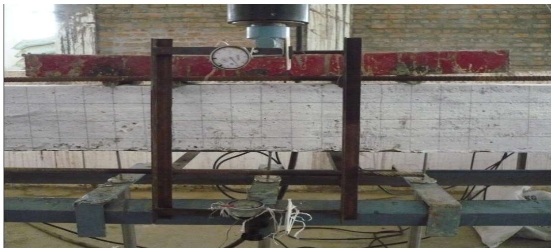
Figure 5: Experimental Setup for the Flexure Beam
