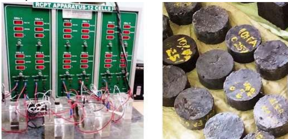
Figure 5. Rapid chloride permeability test
