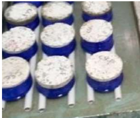
Figure 3.sample being tested for Sorptivity
