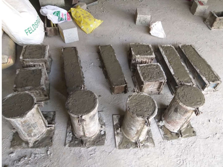
Fig.4. Casting of Specimen
