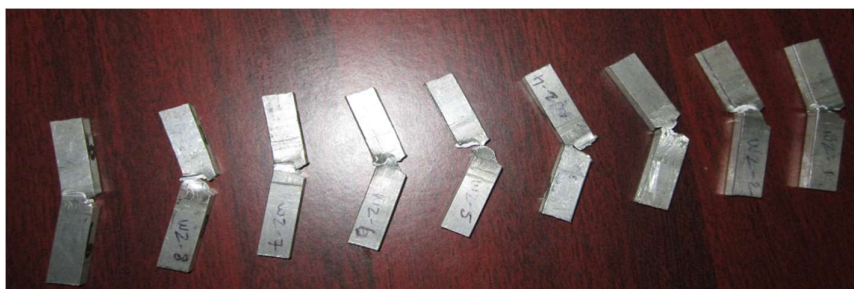
Figure 5. Impact test specimen after fracture
