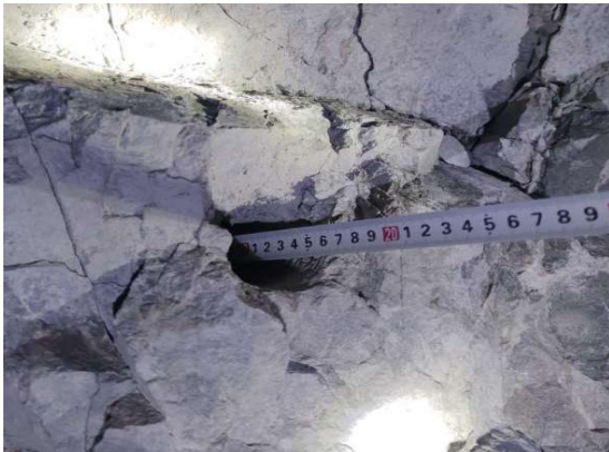
Figure 5. Depth of "shpur residue" in horizontal mine
