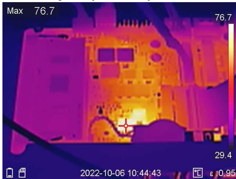
Fig. 2. Temperature distribution on the surface of the motherboard.
