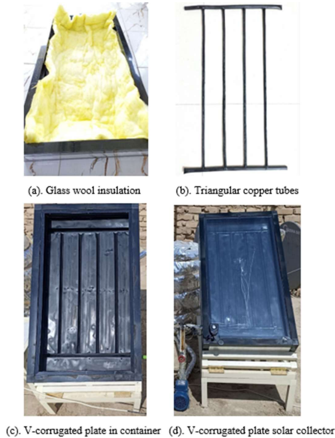
Figure 2: V-corrugated plat solar collector
