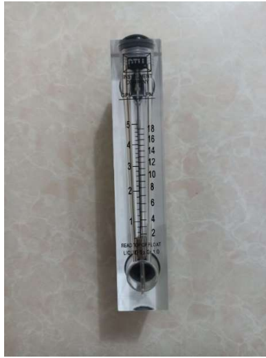
Fig. 5 Volumetric water flow meter
