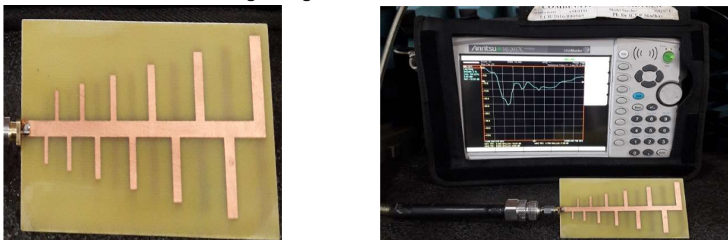
Fig 6. Prototype and measurement setup of the Proposed LPDA
