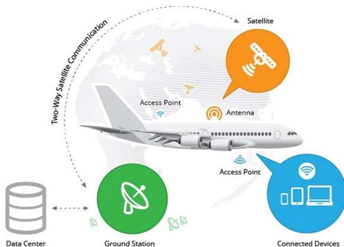
Fig. 2 Scheme of the Internet in an airplane via satellite
