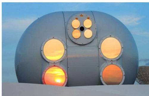
Fig.4 Multi-channel laser communication installation
