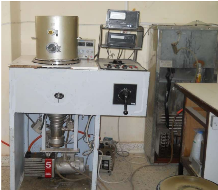
Figure2. The system used in coating samples
