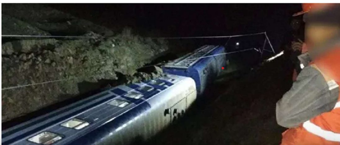
Figure 7. The landslide occurred during the passage of the passenger train No. 081 "Saryasiya - Tashkent", the ground collapse blocked the movement of three cars.
