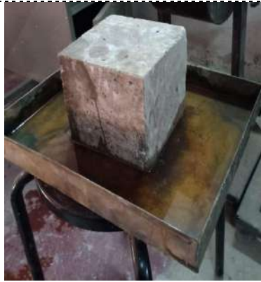
Figure 3. Water Absorption of cubes by capillary action
