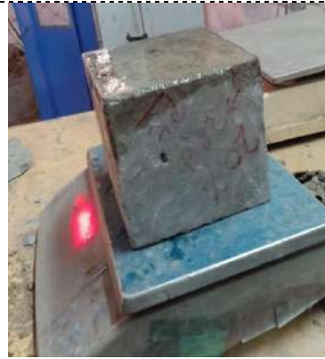
Figure 4. Weighing of cubes after water absorption.
